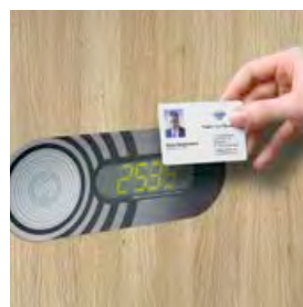
Online locking system with central control unit, with PIN or transponder/data carrier
