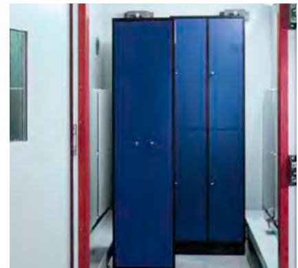
Salt spraying chamber with two lockers which are being tested as a complete product according to DIN 50021 at C+P.
