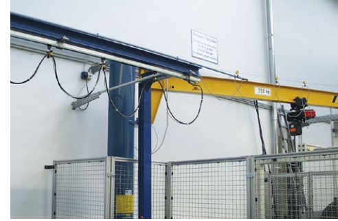
Simple and flexible Festoon System on a C-Rail Track .
