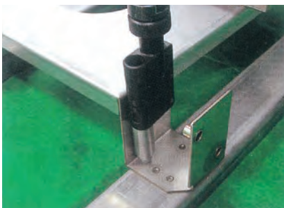
00 Offset nose of AR2000A-00 allows perfect riveting at dead set place
