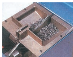
Rivets aligned and sent to the feeder head (with cover open)
