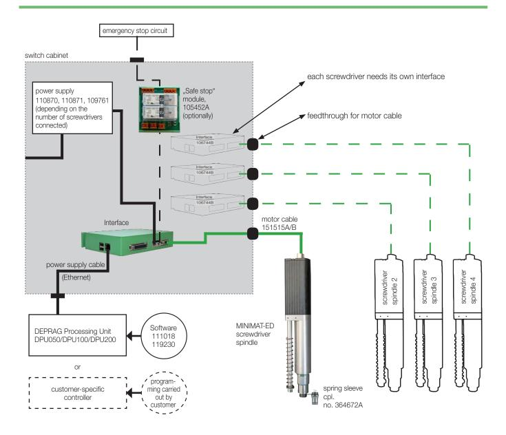
The hardware components required for the adjustment, control and power supply of the screwdriver are intended for integration into a control cabinet.
