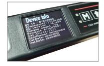
**Tool Compliance** Mitigate or prevent out-ofcompliance use by setting up device with controls on days to next calibration and allowed torque applications
