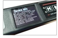
**Tool Compliance** Mitigate or prevent out-ofcompliance use by setting up device with controls on days to next calibration and allowed torque applications
